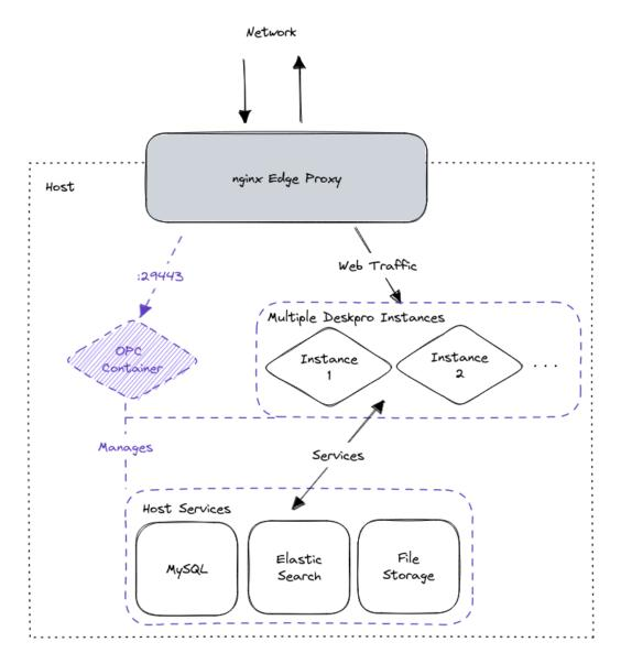
All web traffic accessing the server is handled by the nginx Edge Proxy, but requests made to the special port **:29443** are directed to the OPC container. This container manages the Deskpro instances and the services running within the host. Standard web traffic is forwarded to your Deskpro instance containers, and they can access the required services within the host.
