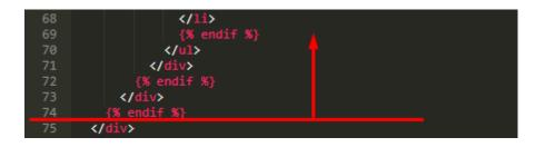
You will notice this is the start and end of the same "if" function. You can also see the same vertical dotted line marking the indentations will align up and connect the first line of the code with the last line. We make use of consistent indentation practices within the HTML to more easily manage the code on the screen, each whole section of code will start and end with the same indentation.
