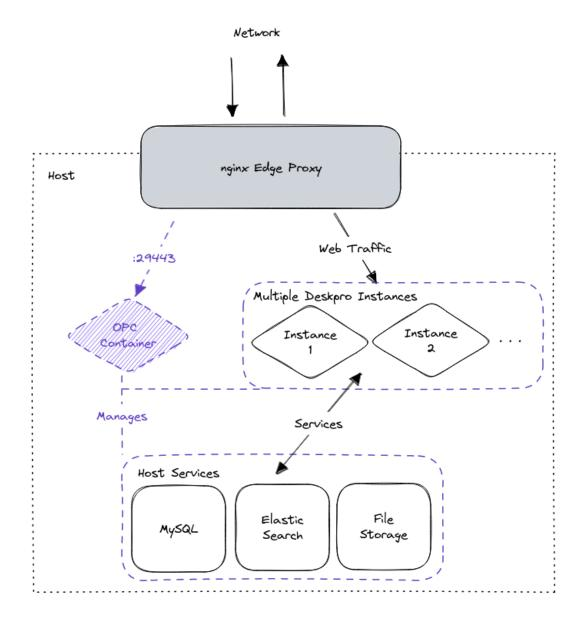
All web traffic accessing the server is handled by the nginx Edge Proxy, but requests made to the special port
